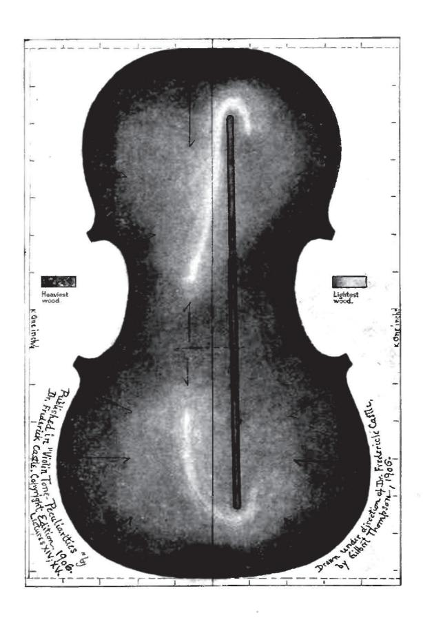
CHART, indicating by shading, the relative quantitive values of violin sounding-board graduation for maximum evenness of tone-power.
